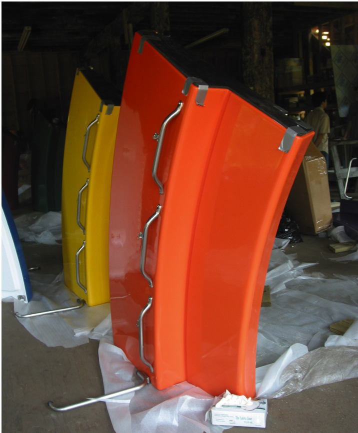
The colorful floating seats are made of fiberglass with stainless steel hardware
