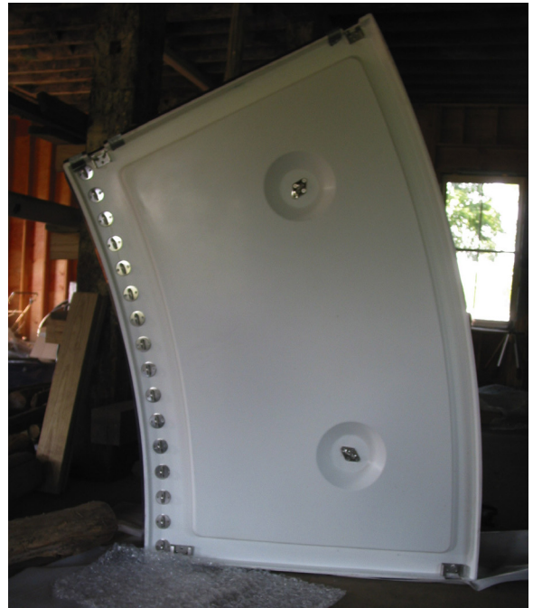
The bottom of the floating seat has recessed hardware
